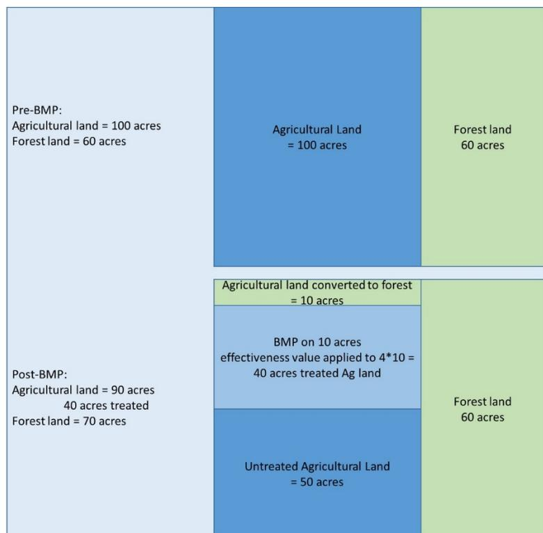
Figure 6-3: Load source change with efficiency example
